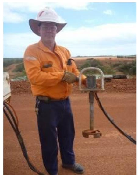
**Figure 2 Hydraulic valve opener tool**
